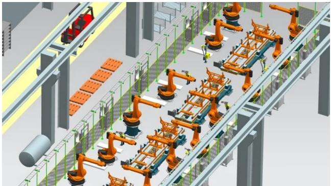
Siemens software includes software to fully design and optimise manufacturing production lines in a virtual environment. Source: <u>https://www.plm.automation.siemens.com/global/en/industries/automotive-</u> <u>transportation/factory-layout-line-design-optimization.html</u>
